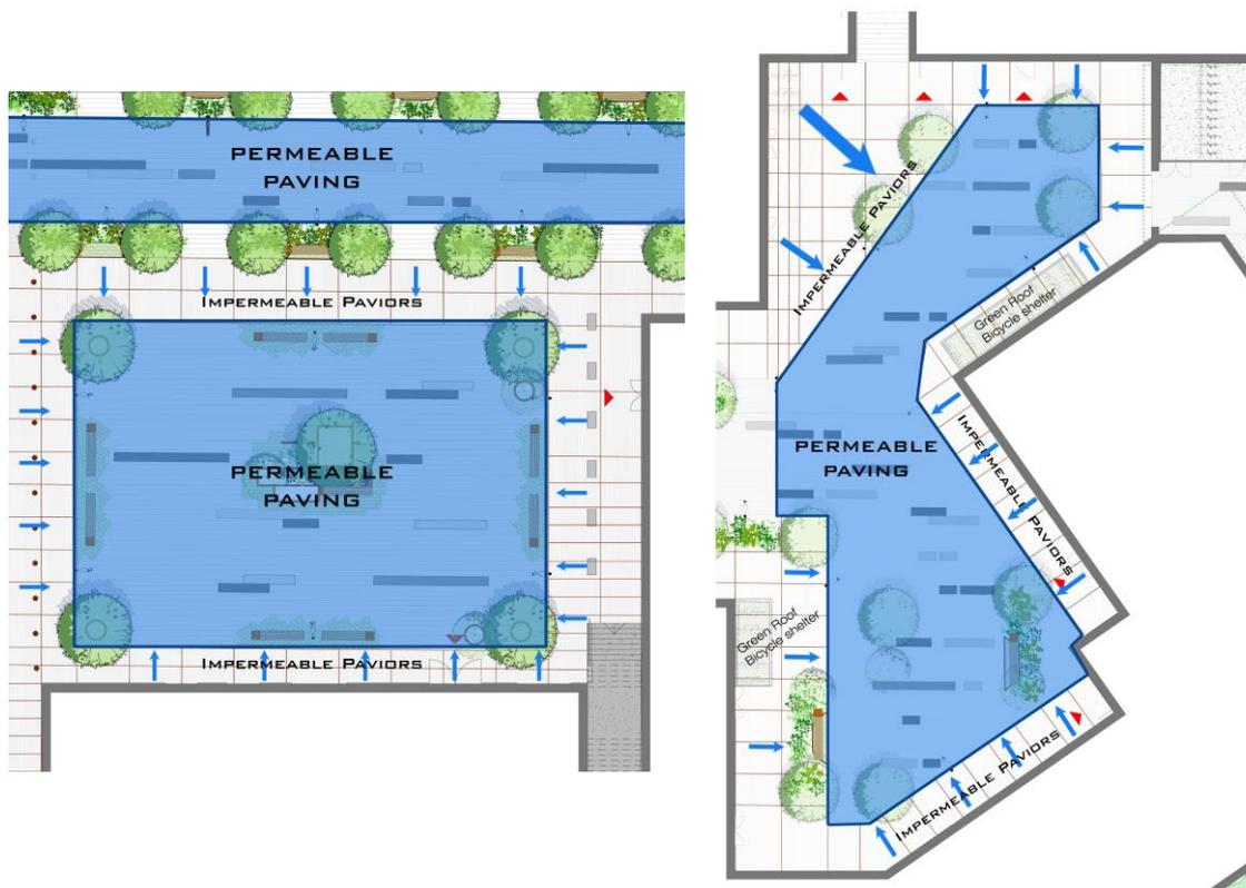
**Figure 5.2** Main areas of Permeable Paving
